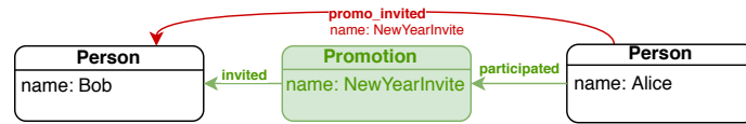
Fig. 3: The edge promo_invited is replaced (red) by the Promotion vertex with two edges (green) by using the Edge to Vertex operator. The Vertex to Edge operator inverts this operation.
